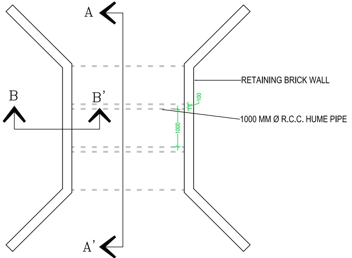
**PLAN OF PROPOSED PIPE CULVERT**
